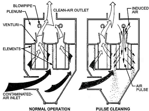
Fig. 14 Pulse Jet Cartridge Filters
